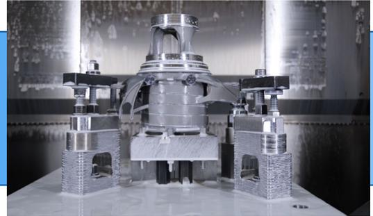
Machining of a "Printed Wheel Carrier
