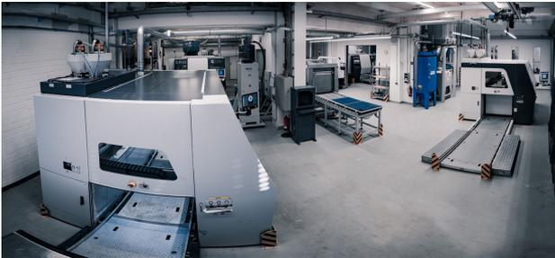
3D printers for sandmolds and cores
